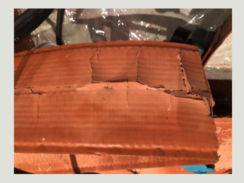
Surface damage from extreme heating and failure of bands
