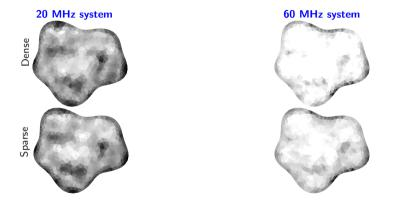
Reconstruction obtained with the total variation (TV) regularisation for the 20 and 60 MHz centre frequencies.
