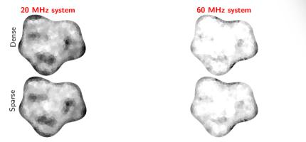
Reconstruction obtained for the TSVD filtered data with total variation (TV) regularisation for the 20 and 60 MHz centre frequencies.
