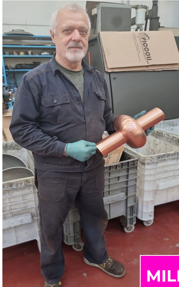
First seamless copper 1.3 GHz cavity produced Courtesy to Davide Piccoli (Piccoli Srl)
