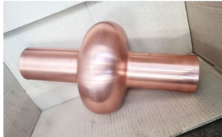
First seamless copper 1.3 GHz cavity produced Courtesy to Davide Piccoli (Piccoli Srl)
