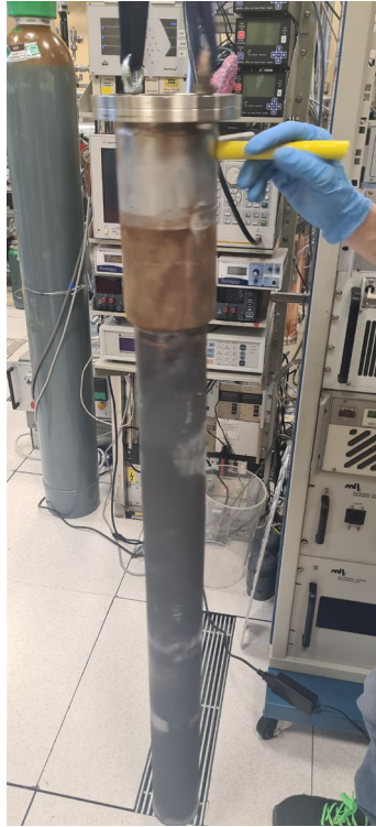
Replacement of old inconel chamber
