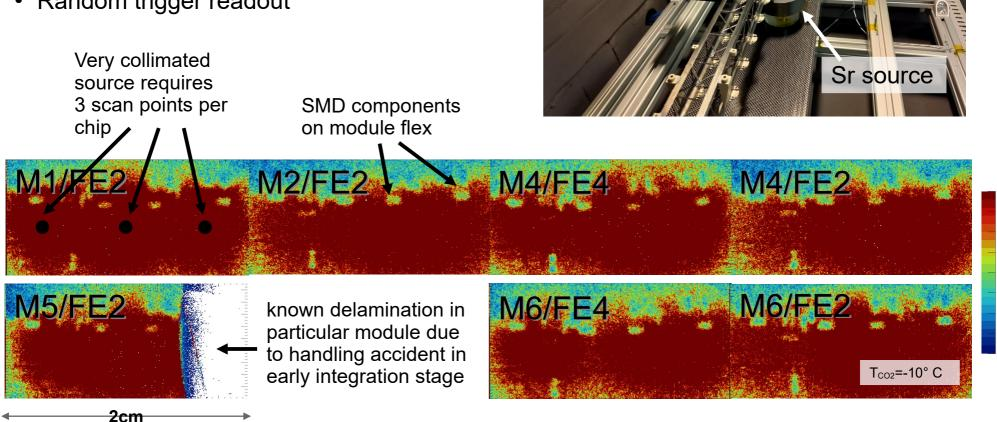
→ No systematic delamination of bump bonds due to loading procedure visible
