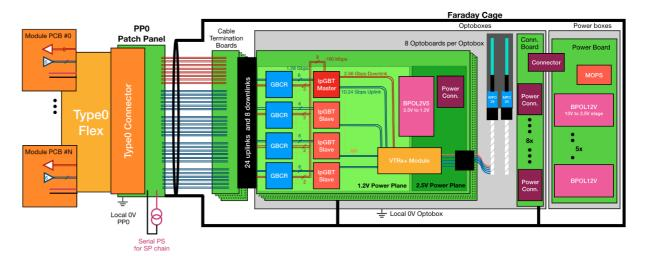
→ Very realistic readout setup and first time large scale validation of opto-system and data-transmission
