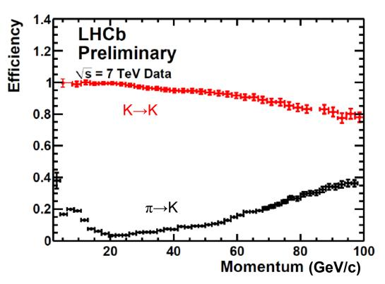
Efficiency / purity working point can be chosen by changing cut value on dLL
