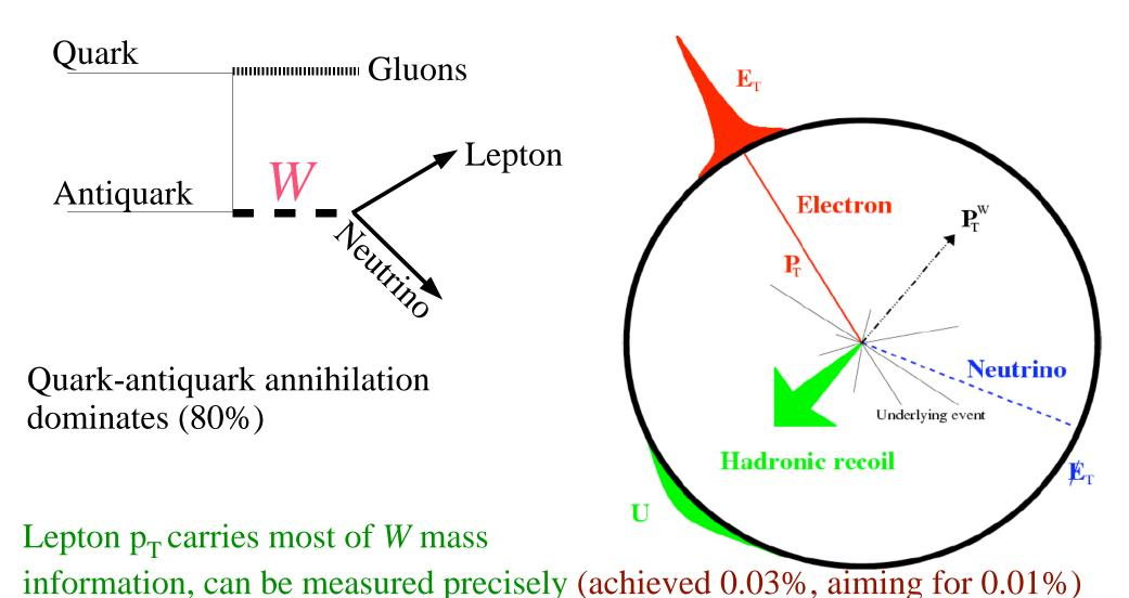
Initial state QCD radiation is O(10 GeV), measure as soft 'hadronic recoil' in calorimeter (calibrated to ~1%, aiming for 0.05%)
