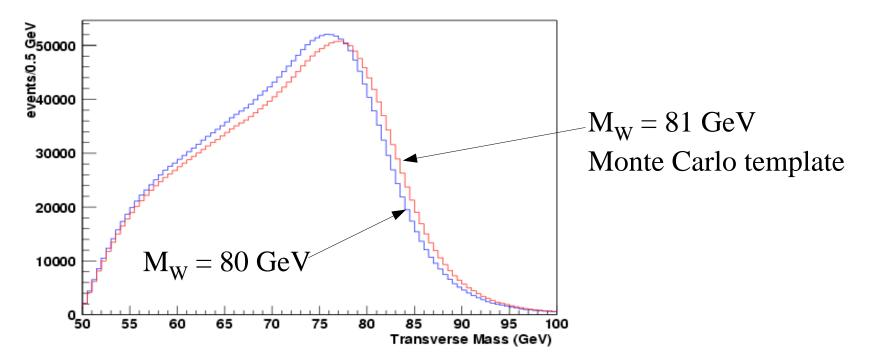
• CDF (and D0) extract the W mass from three kinematic distributions: Transverse mass, charged lepton  $p_T$  and neutrino  $p_T$ : different recoil systematics
