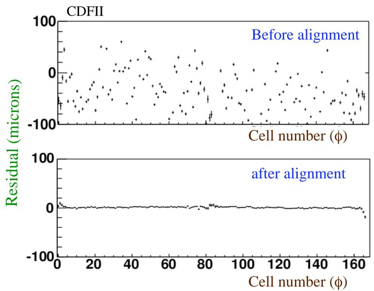
Final relative alignment of cells ~5 μm (initial alignment ~50 μm)
