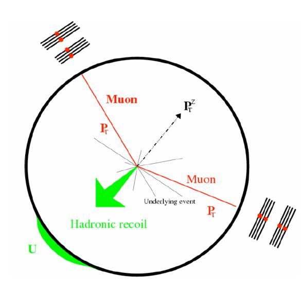
Transverse momentum of Hadronic recoil (*u*) calculated as 2-vector-sum over calorimeter towers
