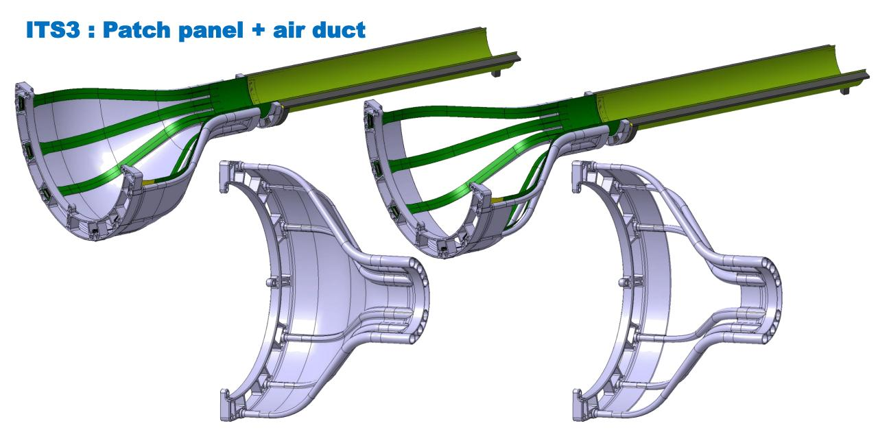
Full shell = rigid link between half ring and patch panel
