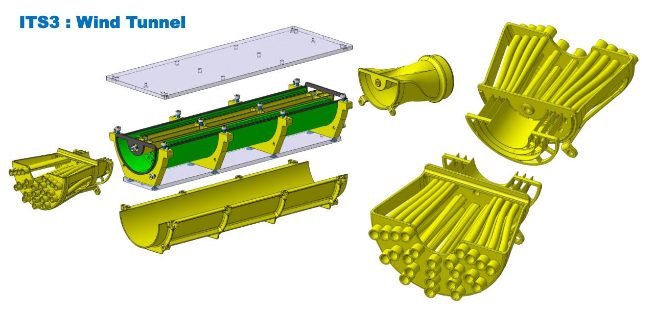
Different air pipes configuration possible for each layers
