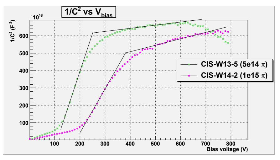
Depletion voltages from CV(-25C, 55 Hz) and IV:
