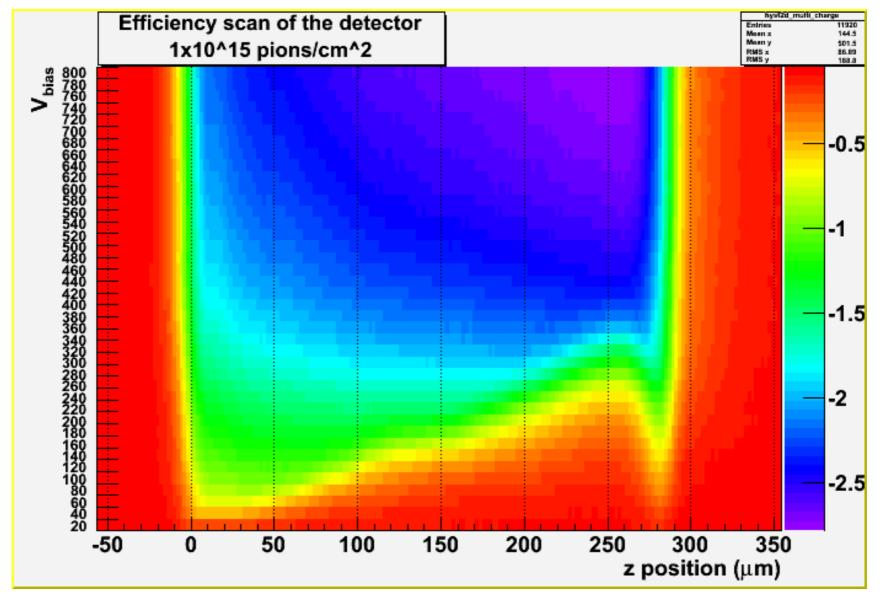
Again, more efficiency in the back region at high voltages. Trapping is influencing less carriers generated in this region (might be due to higher drift velocity of electons that have anyway lifetimes comparable to holes)
