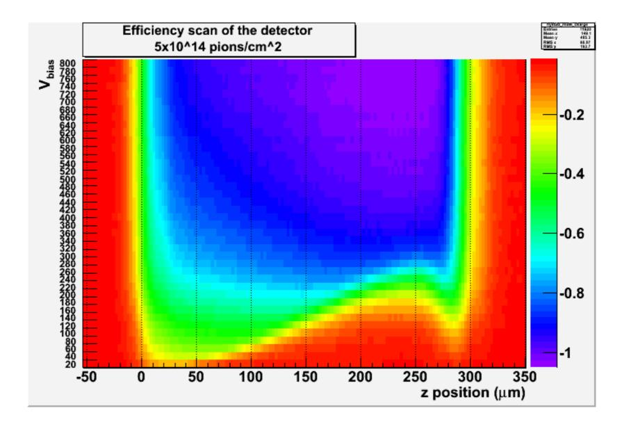
Back of the detector becomes more efficient than front region at high voltages
