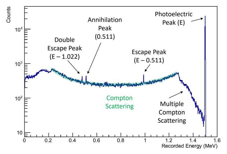
Line widths are usually set by the resolution of the detector. Germanium detectors have resolutions of 1 to 3 keV.
