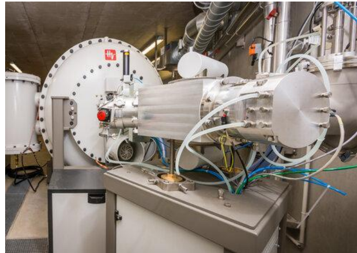
3.5 MeV e-beam Accelerator Source: ATRON
