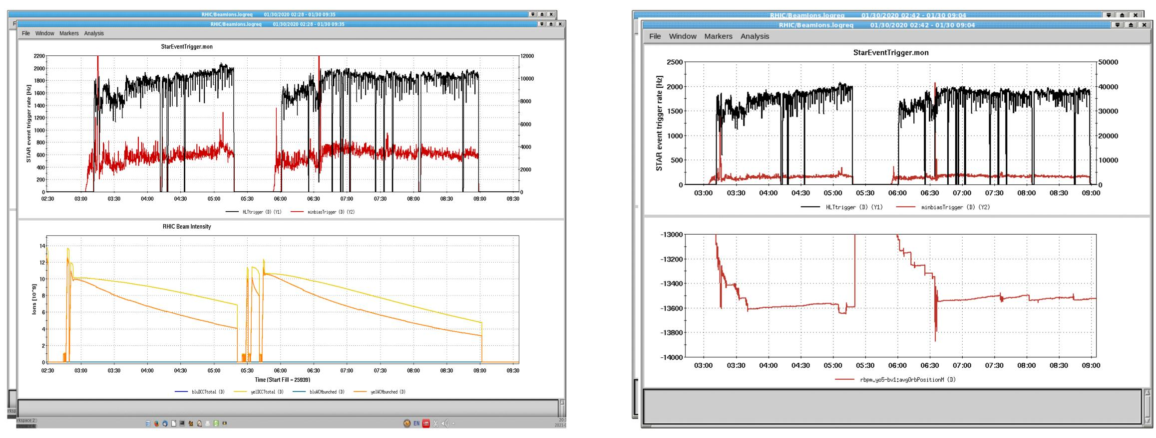
The upper plot shows the fixed target event rate (in black) and minbias rate (in red) over the time period of two physics stores at 9.8 GeV. The lower plot shows the beam intensity evolution during the stores, total beam intensity in light yellow and bunched beam intensity in dark yellow.
