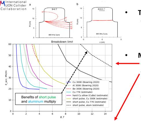
Model developed by US labs, checked against measurements in high *B*. Papers: Palmer et.al PRAB 2009, Stratakis et.al NIMPR 2010, Bowring et.al PRAB 2020
