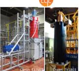
Frequency: 1.0 GHz Peak RF power: 20 MW Efficiency: 70%
