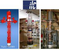
Frequency: 1.3 GHz Peak RF power: 10 MW Efficiency: 65%
