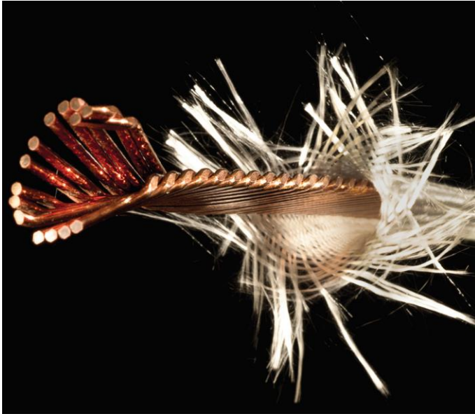
Nb 3 Sn cable for high-field accelerator dipole and quadrupole magnets
