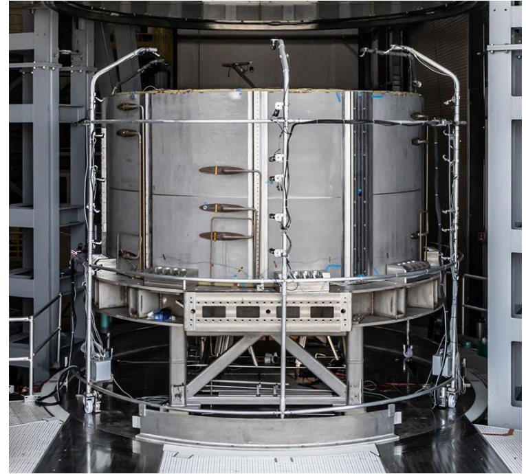
ITER Central Solenoid, 13.6 T, 2 m \text{Nb}_3\text{Sn}
