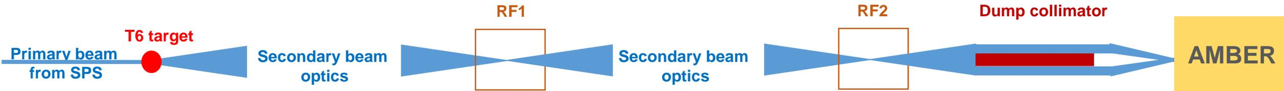
Parallel optics: Minimize beam divergence in the cavities
