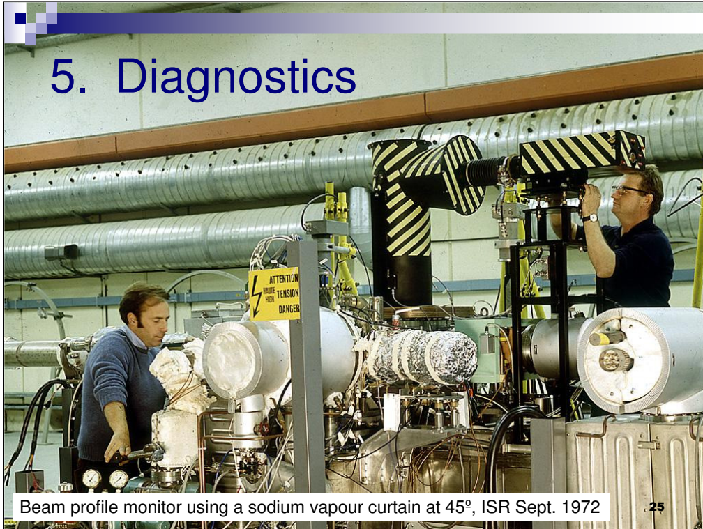
Beam profile monitor using a sodium vapour curtain at 45 degrees.
