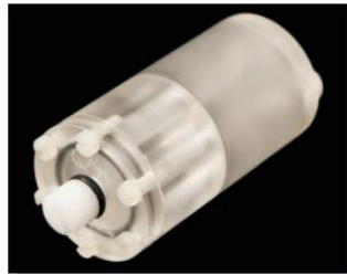
Micro-PET IQ Phantom (according to NEMA NU 4-2008)
