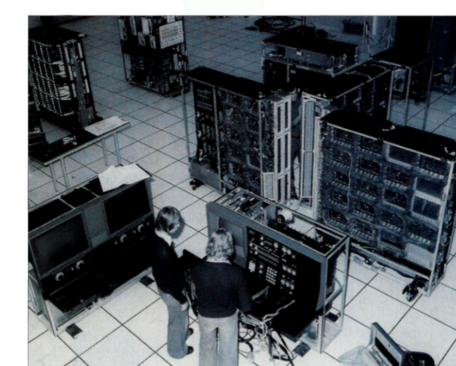
The arrival of the IBM 370/168 in 1976 ushered in the heyday of the mainframe and the "CERN unit" of physics data processing.
