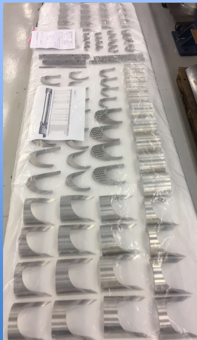
4 sets: Ti poles and spacers, SS saddles
