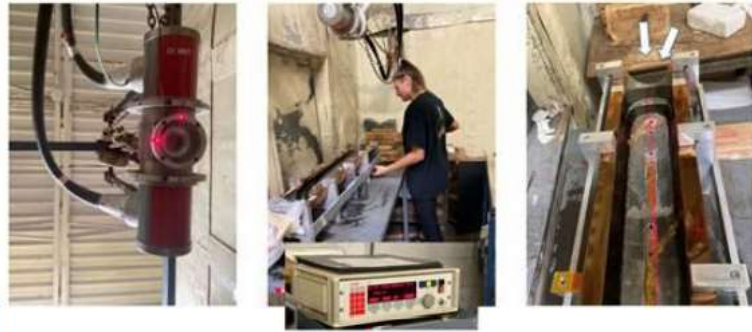
300 kV CT scan at AlloyWeld Inspection (Illinois)
