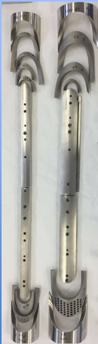
4 sets: Ti poles and spacers, SS saddles
