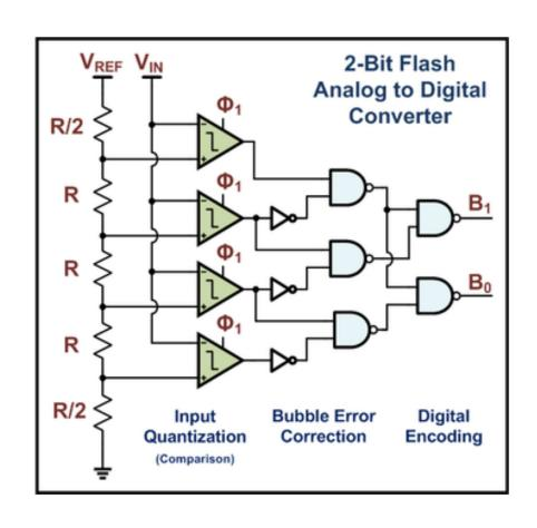
A Flash ADC can digitize a signal very fast without a clock
