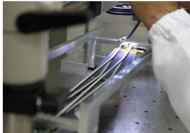
Pulling the problematic wirebond
