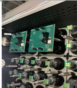
Step C: Attaching FEE (Pogo Pins, utilizing existing holes in EM Module)
