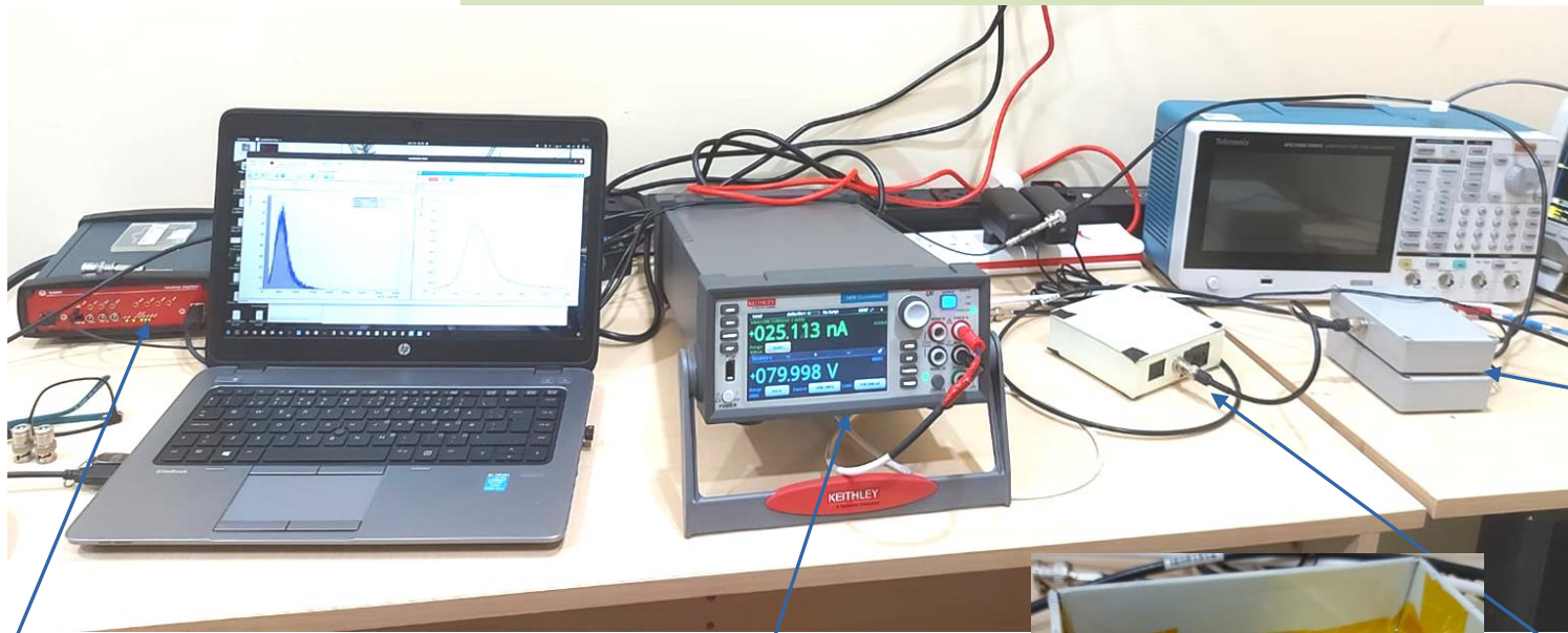
CAEN Digitizer (DT5730) 8 ch, 14 bit resolution, 500 MS/s sampling rate, 2Vpp dynamic range
