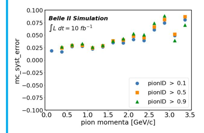
$mc\_syst\_error$  is observed to increase in bins of momenta with the maximum difference being about 7.5%.
