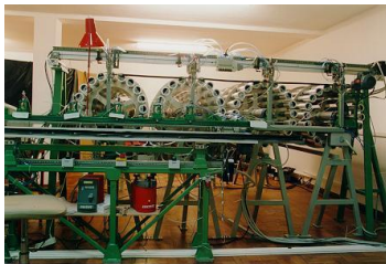
Robot for fiber insertion. 600 000 fibers inserted in Lisbon and later in Coimbra
