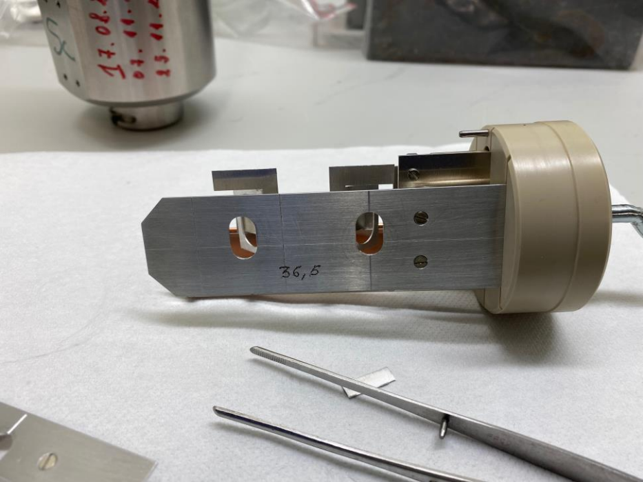
Fig. 24. Collection chamber for double collection with reduced sputtering
