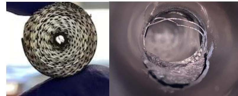
Fig. 12. Intact (left) and molten (right) Ti roll target material.
