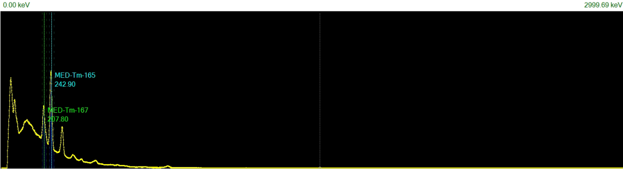
Fig. 26. Kromek \gamma -spectra during double beam collection of Tm-165 and Tm-167 simultaneously
