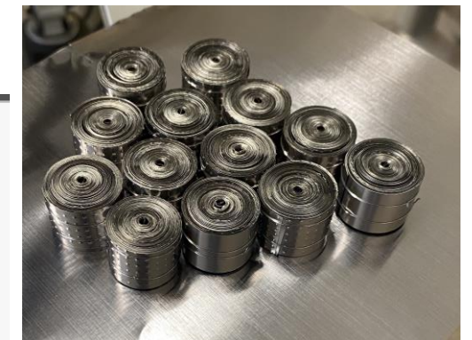
Fig. 20. natTi double rolls used for Sc radionuclide production
