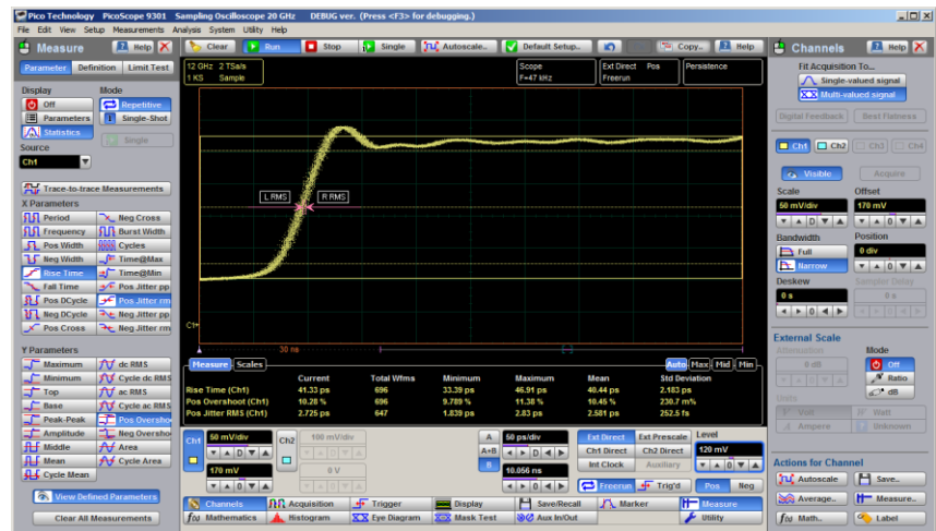
40.44 ps step rise time having 2.48 ps RMS jitter
