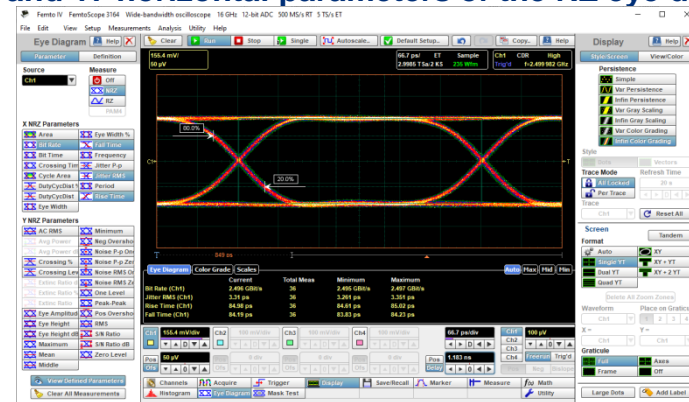
Disclosed 2.5 Gb/s eye diagram
