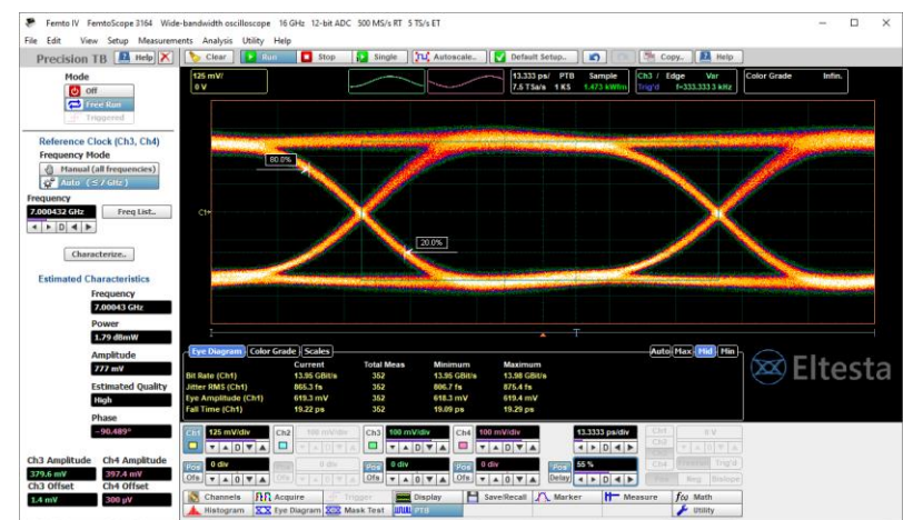
14 Gb/s eye diagram acquired with precision time base of the FemtoScope 3164-PTB shows 875 fs eye RMS jitter.
