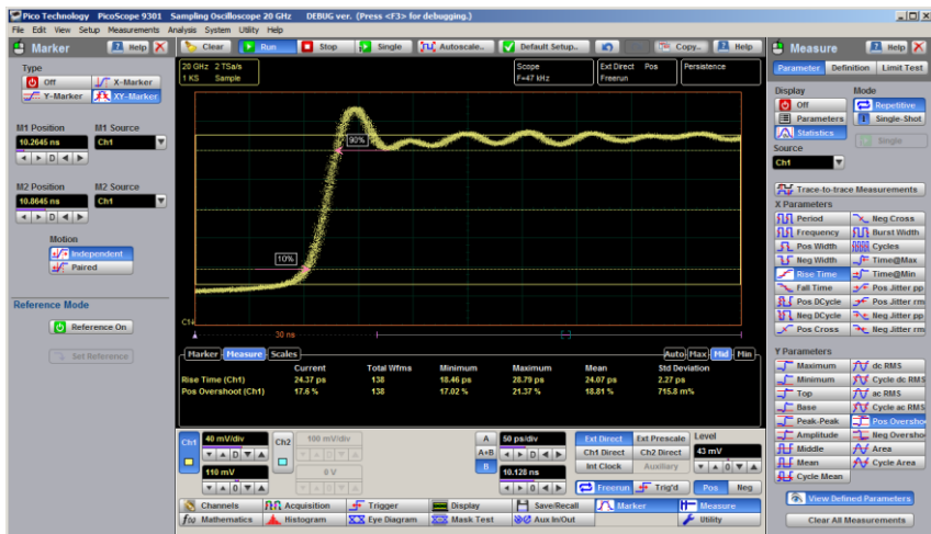
Transient response shows 24.07 ps step rise time and 16.84% overshoot
