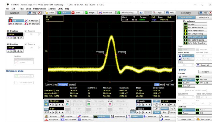
The FemtoScope 3164 demonstrates internal direct trigger from pulse having 35.3 ps width and 98 mV amplitude. Signal source: Anritsu MP1800A Signal Quality Analyzer
