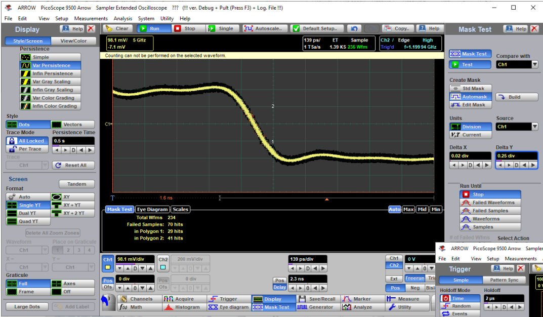
Automask measurements of a pulse having 150 ps fall time
