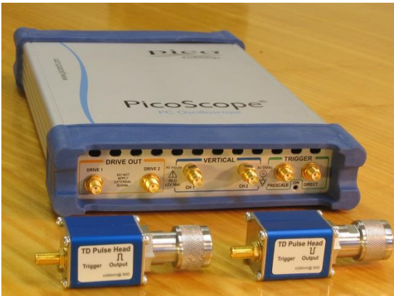
The PS9321: Dual-channel, 20 GHz bandwidth with 35 ps rise time / 200 mV TDR/TDT differential pulse generator
