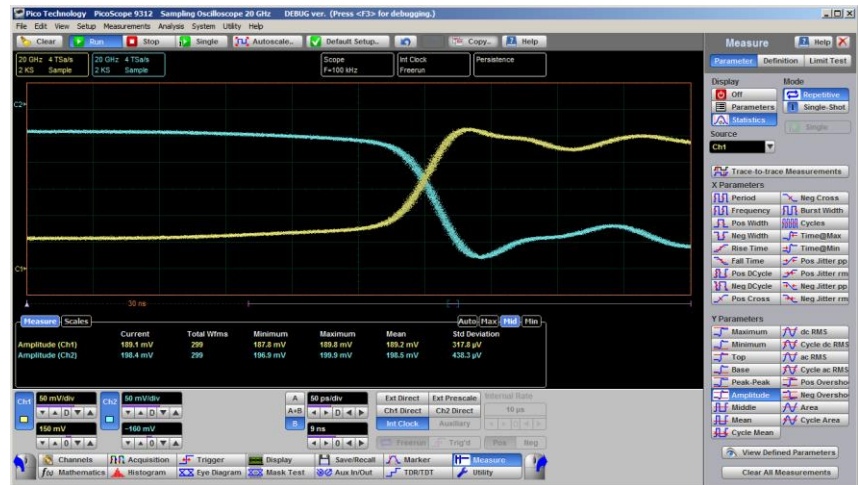
35-ps differential steps at 50 ps/div time base
