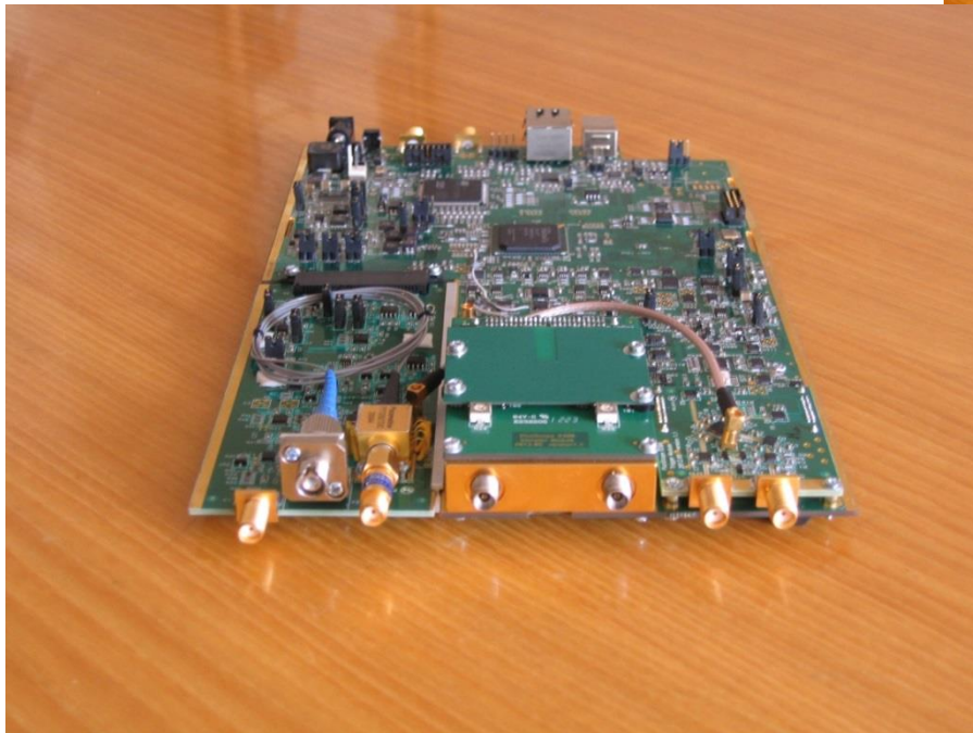
Acquisition Board with Dual-channel Sampler and Trigger modules, also with optical/CDR module
