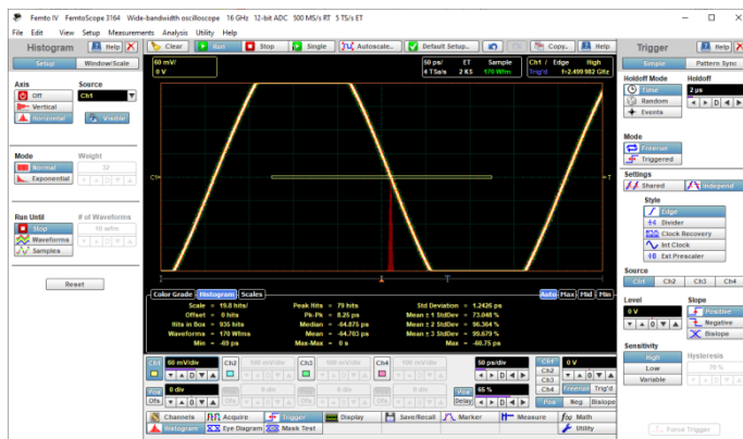
Internal direct trigger from 2.5 GHz sine wave with 1.24 ps rms jitter.
