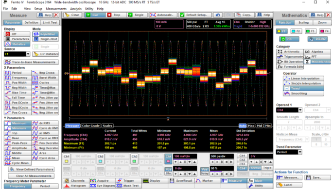
Trend of period measures nonlinearity of oscilloscope time base with 5-GHz sine wave. Maximum trend of period = 202.5 ps. Minimum trend of period = 197.8 ps. Peak-peak nonlinearity is within +2.5/-2.3 ps at 5 ns timing window
