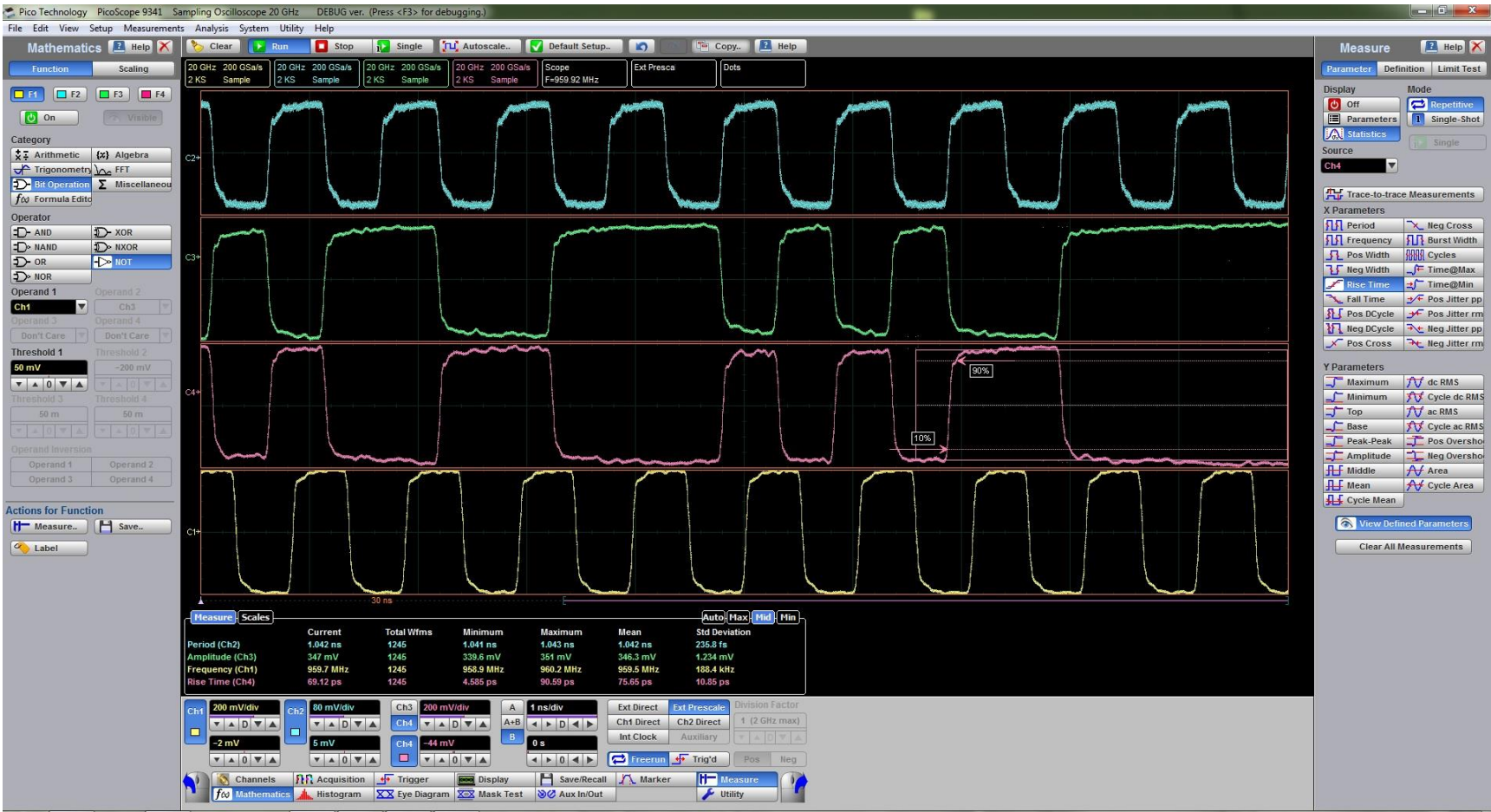
1 Gbps patterns and clocks on 4-channels PicoScope 9341 sampling oscilloscope
