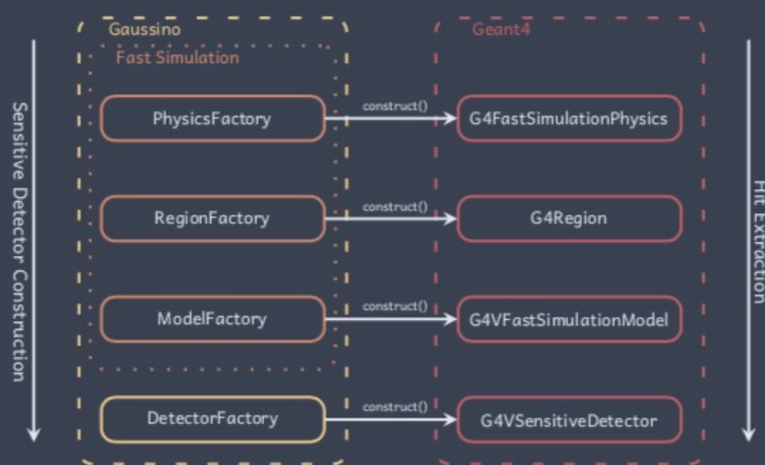
Figure: A simplified model of the FastSimulation interface with a set of dedicated factories that construct the corresponding Geant4 objects.
