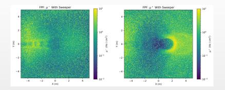
$\ast$  BDSIM simulations on a 4  $\times$  4 m<sup>2</sup> area transverse to the LoS at 617 m from the ATLAS IP, including sweeper magnet effects, for the nominal HL-LHC integrated luminosity.
