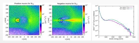
\* FLUKA simulations on a 4 x 4 m<sup>2</sup> area transverse to the LoS at 348 m from the ATLAS IP, for the nominal HL-LHC integrated luminosity.
