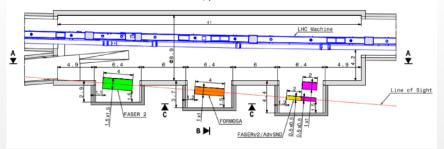
The LoS touch marginally UJ12. One could envisage to enlarge UJ12 to better encompass the LoS, with alcoves for different experiments.
