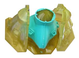
WE DECIDED TO DESIGN A MOULD IN ORDER TO PRINT THE MOULD INSTEAD OF THE MASK, AND PRODUCE SEVERAL MASKS BY MANUAL INJECTING SILICON
