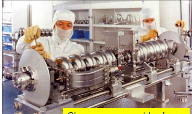
Clean room assembly of superconducting RF cavities
