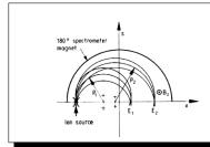
Mass spectrometers entirely rely on weak focusing: they have no quadrupoles; particles are separated according to their energy and focused due to the  $1/\rho$  effect of the dipole
