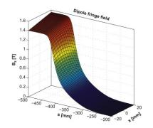
Fringe field of a dipole magnet (in this case: a combined dipole + quadrupole magnet, notice the slope of the field along the x axis)
