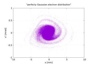
An initially Gaussian electron bunch, *filamenting* after traveling through the CLIC Drive Beam Recombination Complex, under the effects of non-linear fields, chromaticity, and synchrotron radiation.
