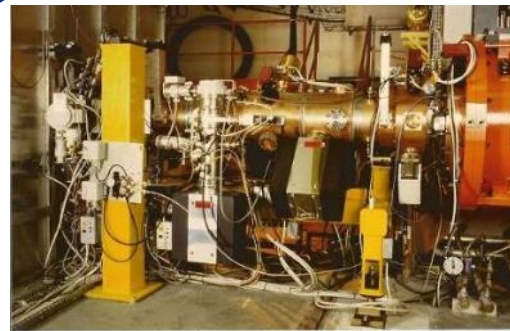
The new RFQ2 pre-injector at CERN (1993): Source+LEBT+RFQ
