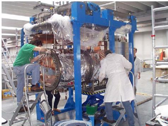
At prototype and the final installation of the superconducting RFQ at LNL, Italy
