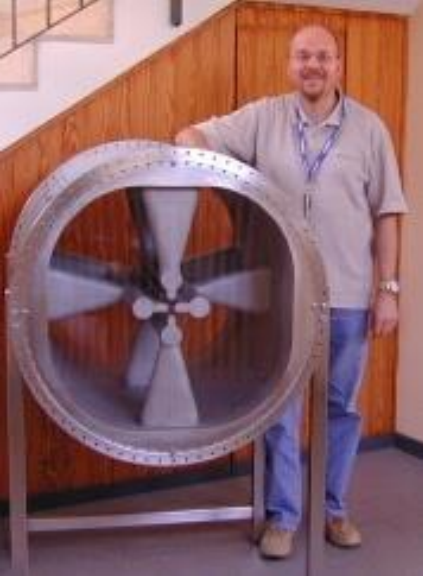
At prototype and the final installation of the superconducting RFQ at LNL, Italy
