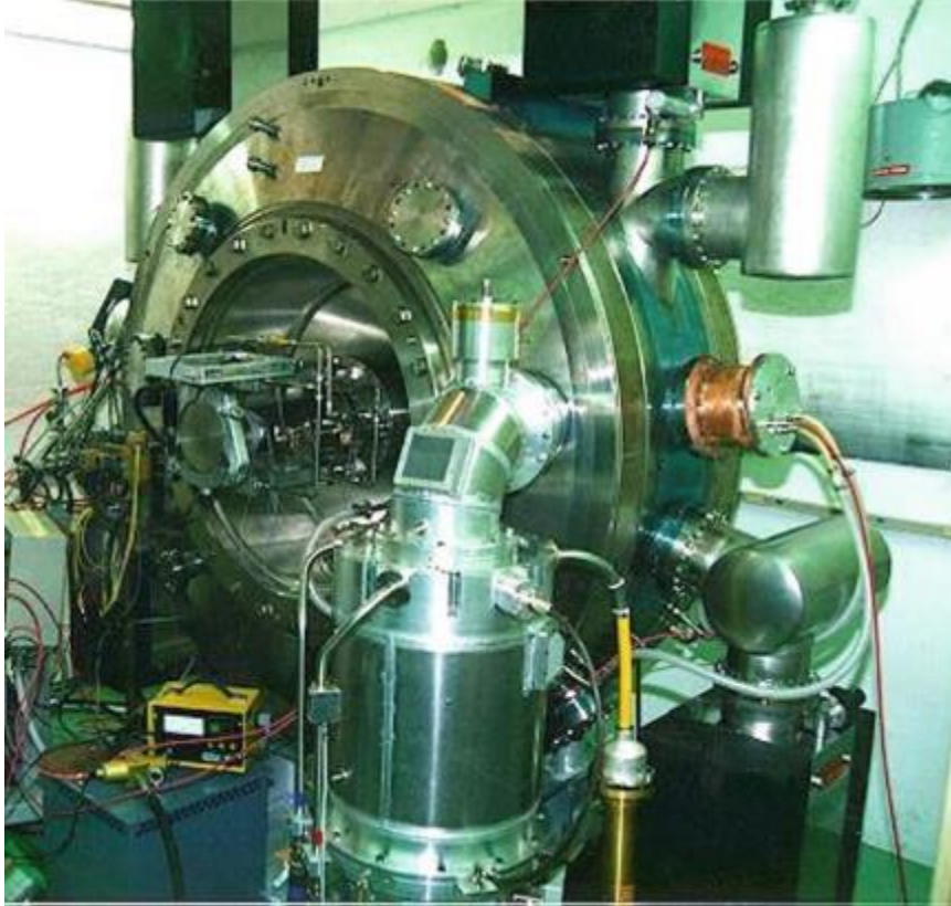
The pillbox becomes quite complex... CERN PS 80 MHz cavity (for LHC beams)
