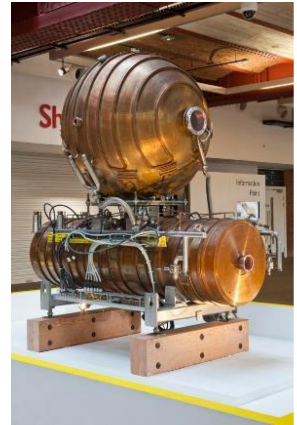
One of the 16 cavities installed in the old LEP collider: 352.2 MHz, 5 coupled cells, equipped with a spherical storage cavity on top to reduce losses
