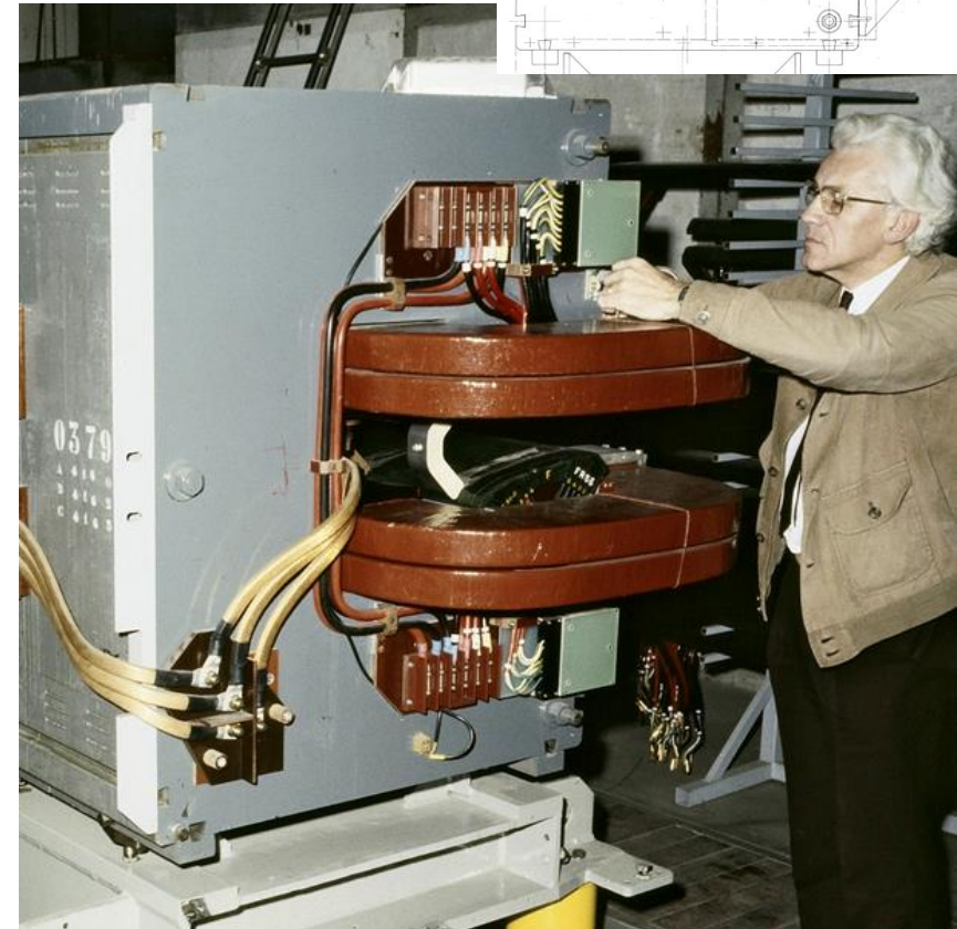
One of the dipole magnets of the PS, in operation at CERN since 1959
