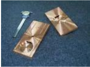
The LIBO prototype structure and accelerating cells (CERN)
