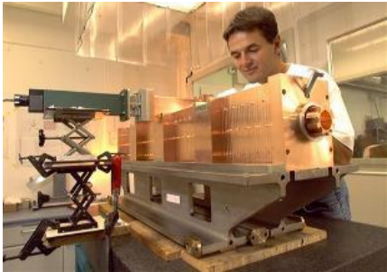
The LIBO prototype structure and accelerating cells (CERN)
