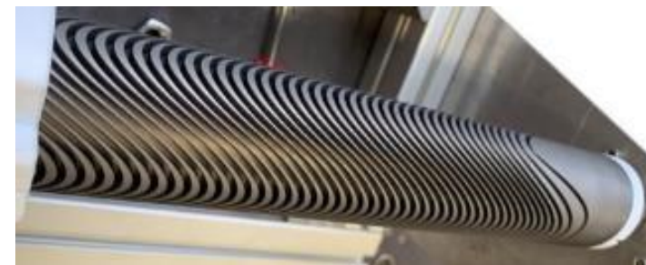
Solution for curved and straight CCT coils combining dipole and quadrupole in the same winding - Courtesy G. Kirby and J. van Nugteren, CERN
