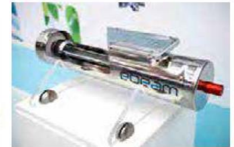
Fig. 4.13: Tetra Pak has a new generation of automated filling machines that uses e-beams to sterilise packaging.
