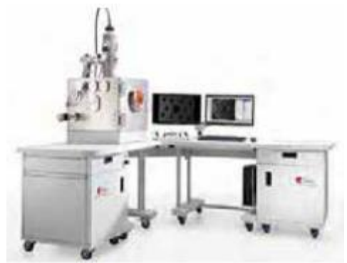
Fig. 4.8: A desk-top e-beam laboratory machine for welding and structuring with a magnified backscattered electron-image.
