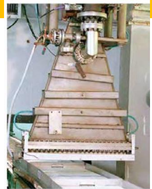
Fig. 4.12: E-beam technology for sterilising medical products
