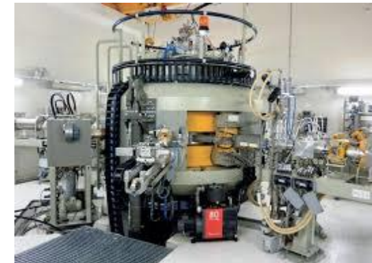
Proton cyclotron for radioisotope production
