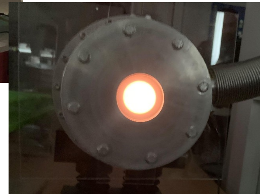
The obtained beam image from the fluorescent screen placed at the end of the PM-MDIS system.
