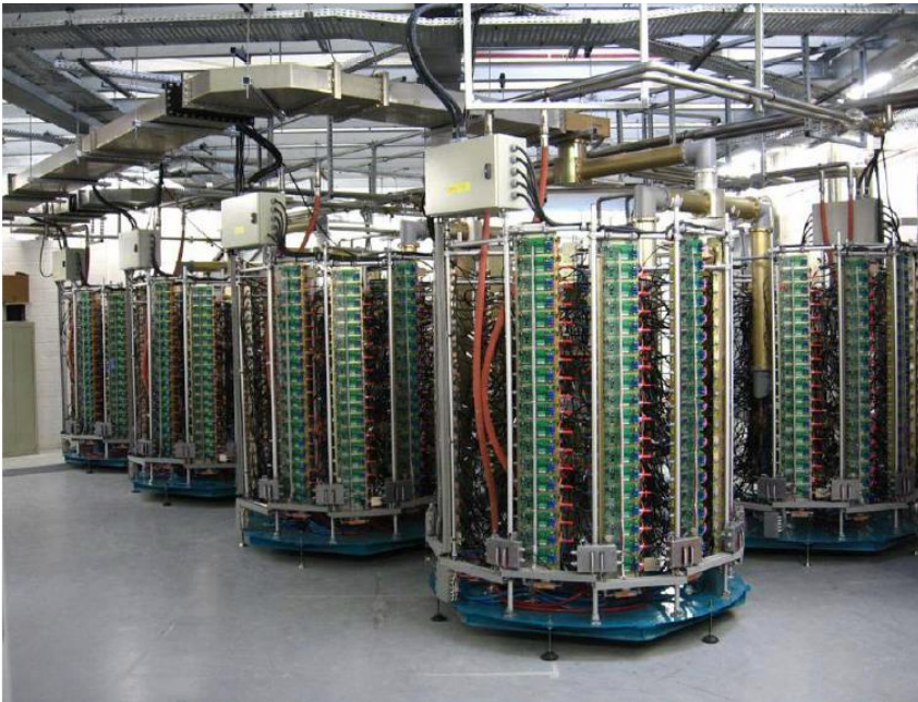
SOLEIL 45 kW @ 352 MHz solid state amplifier towers (2004 & 2007)
