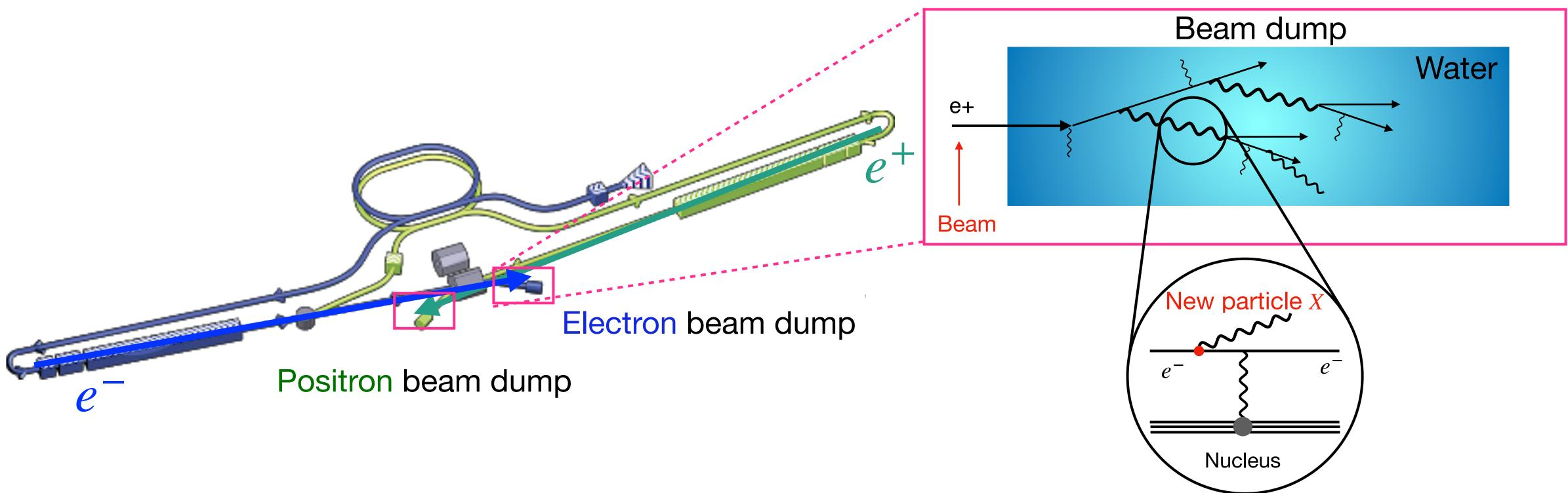
Linear Collider Experiment ⇒ After beam collisions almost all beams are discarded in main beam dump \* To avoid radiation contamination ILC-250  $\Rightarrow$  Energy in Lab frame: 125 GeV, Flux: 4  $\times$  10<sup>21</sup>/year The discarded beams can be converted into new particle beams
