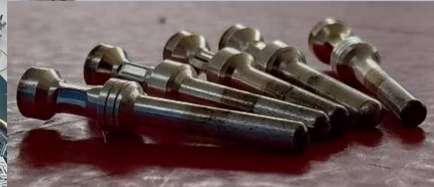
Harting pins after few thousand mating cycles
