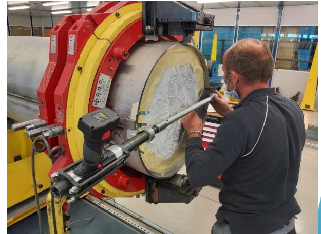
Stainless steel shape re-rounding using a jack in the extremities
