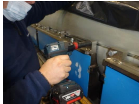
Upper shell tight adjustment to the magnet yoke and backing strip
