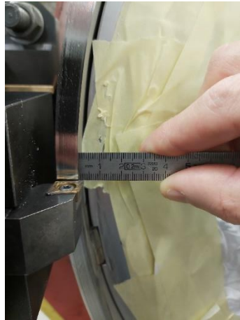
Shells elliptical shape in the extremities
