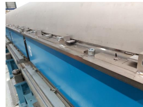
Upper shell sitting on top of the shims surface
