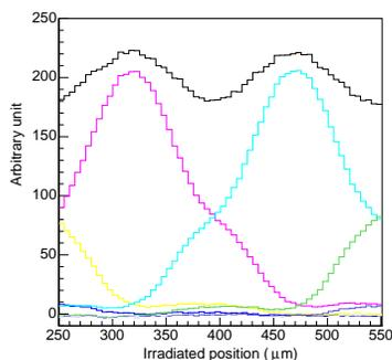
Fig. 4. Charge of readout signals for each strips and their sum as a function of irradiated position by infrared laser.
