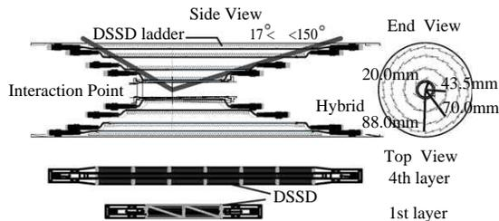
Fig. 1. Mechanical structure of the SVD2 detector.
