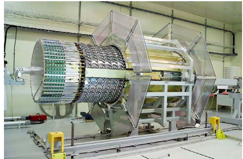
Outer barrel being inserted in outer thermal enclosure
