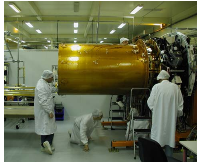
Outer thermal enclosure fitted – ready for insertion into TRT
