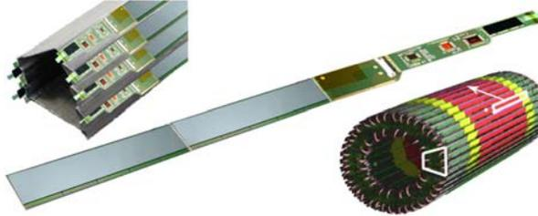
Fig. 1: Artistic view of the components in a half stave, of one sector and a CAD drawing of the SPD.
