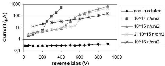
Fig. 2. Current-Voltage characteristics of “n-in-p” microstrip detectors irradiated with neutrons. The measurements (26) have been performed at a temperature of  $-30^\circ\text{C}$ .
