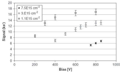
Fig. 1. Charge collection efficiency versus applied voltage, normalized to pre-irradiation value, of “n-in-p” strip detectors (vertical scale is in Ke). The radiation fluences (in p/cm<sup>2</sup>) are shown on the left box. The detector irradiated at  $3 \times 10^{15}$  p/cm<sup>2</sup> is a standard p-type substrate, while the others are oxygen enriched. The measurements (8) have been performed at a temperature of  $-20/25^\circ\text{C}$ .
