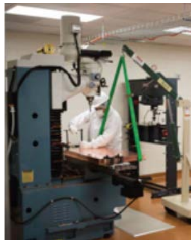
Copper being electroformed on a stainless steel mandrel
