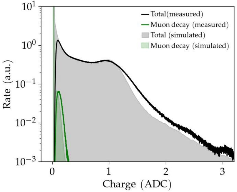
The integral of the time trace results in the total charge collected at the PMT. A comparison between the
