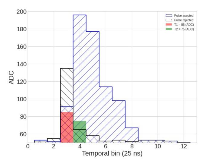
trigger levels searching for expected two exponential behavior of time difference histogram of signal in the WCDs (from secondary cosmic radiation and muon decay inside WCDs)
