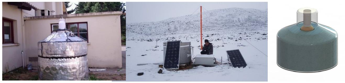
other in Peru's Antarctica Camp (ANTAR, center). The Cherenkov light produced in purified water by air showers entering the detector is measured by a 9" photomultiplier tube (PMT) centered at the top of the detector (right).
