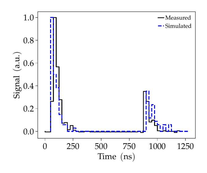
We performed simulations in order to compare the results with the measured data. The response of a WCD to the flux of secondary particles was simulated Geant4. A using comparison between a **measured** and a simulated time trace of a decayed muon is shown in the left.
