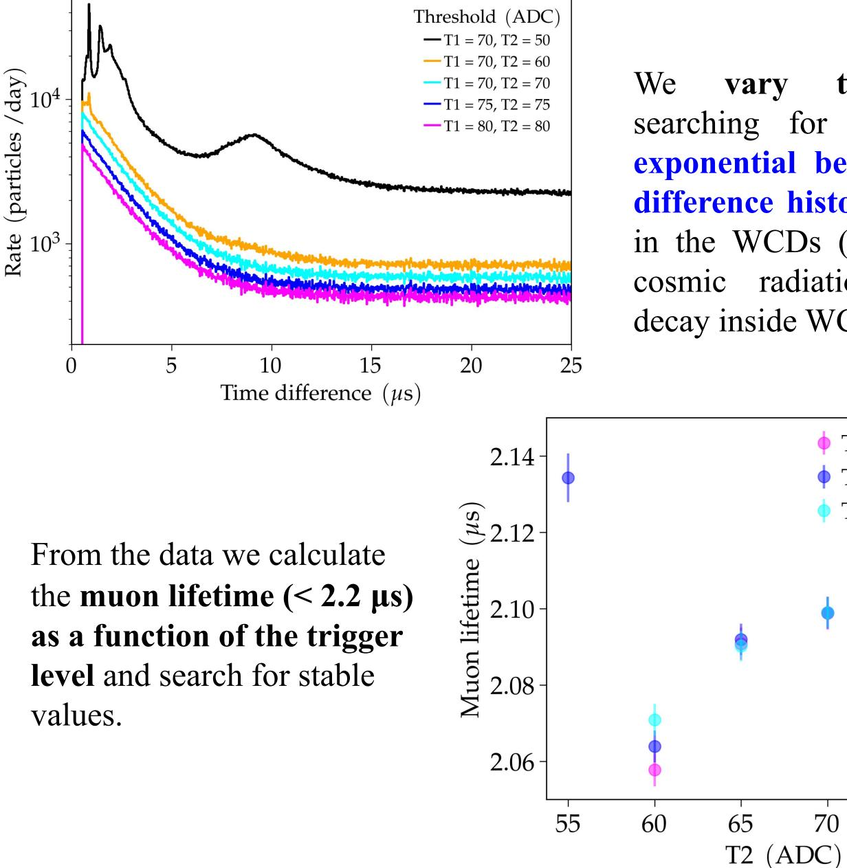
Sources of noise in a LAGO's WCD come from light leakage, electronic noise, thermionic emission and after-pulses; noise signals are expected to present a short pulse width (few nanoseconds) and characteristic differential time spectrums 25 signal below 5 μs.
