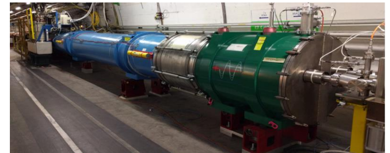
BSRT light sources – undulator magnet (green) and dipole magnet (blue)
