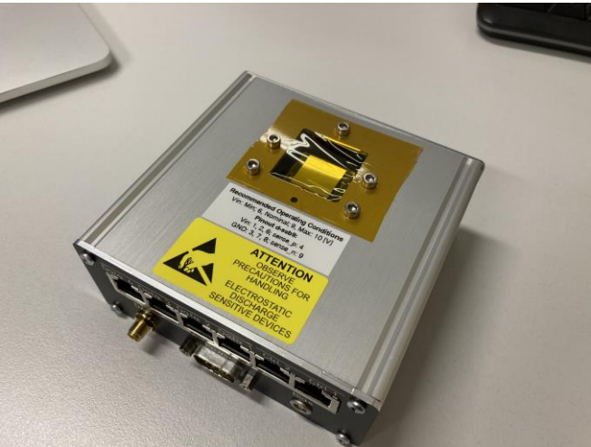
Radiation tolerant Fast BLM based on Timepix3 with BIPXL readout
