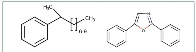
**Figure 2**: Structural formulae of the two primary components of the SNO+ scintillator cocktail. Left: LAB is a phenyl group attached to a carbon chain varying between 9–14 (>95% 9–12) carbons in length. Right: PPO is the fluorophore of the liquid scintillator cocktail.
